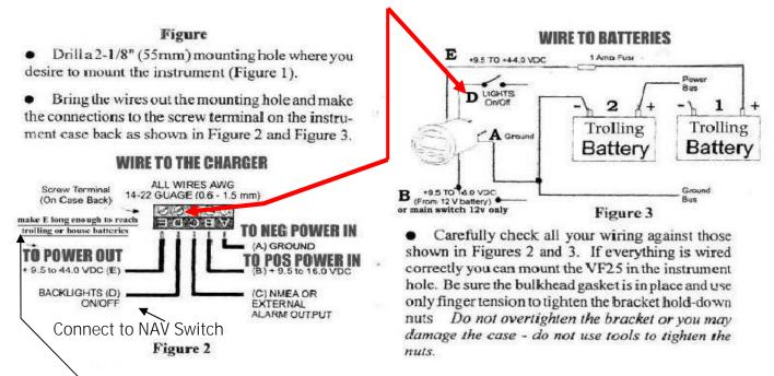
Again leave enough wire from E to reach the charger and trolling or aux Batteries. Also if E is connected to the Page 6 Stealth DC power out post put it on under the nylon nut for easy finger removal.Page 7
